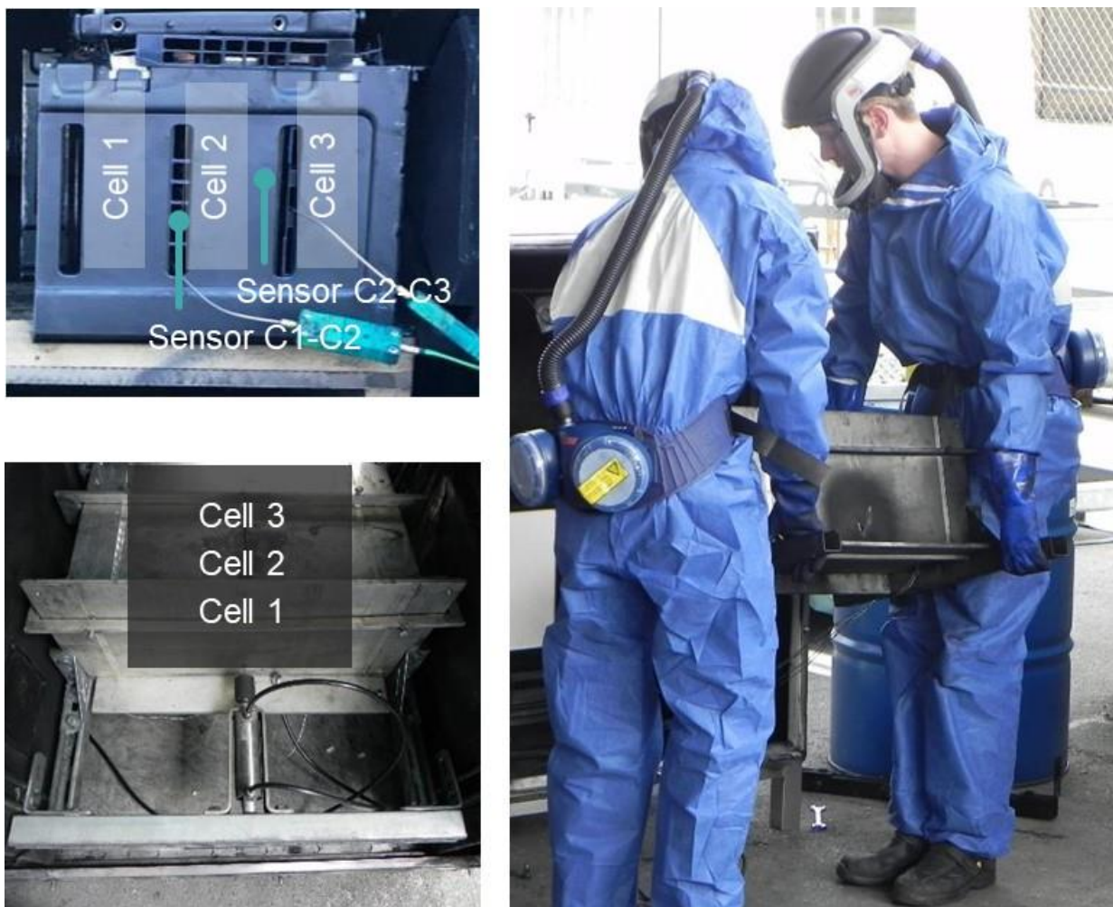
Figure 10: test setup runaway propagation
